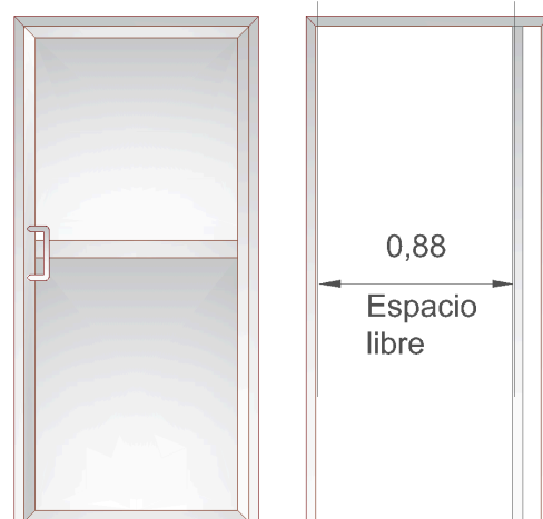
*Clearance for door of 2.20m x 1.00m
