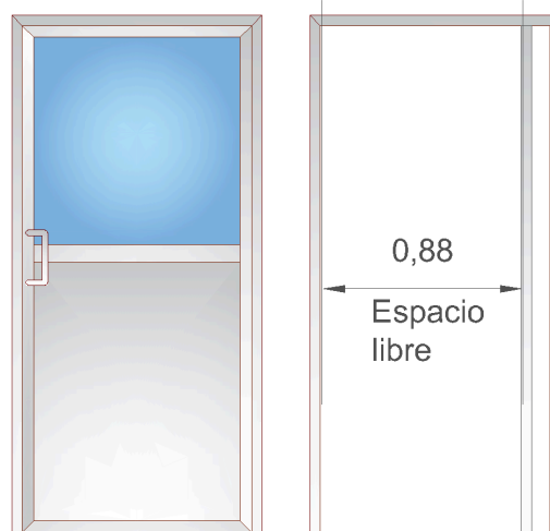
Clearance for a door of 2.20m x 1.00m
