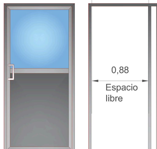
Clearance for door of 2.20m x 1.00m
